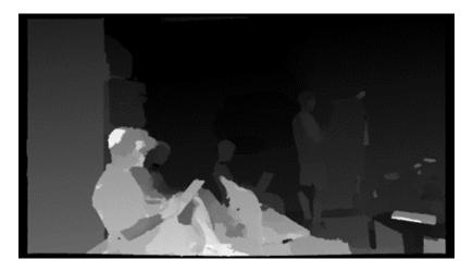
Depth map acquired by Kinect depth sensor:
