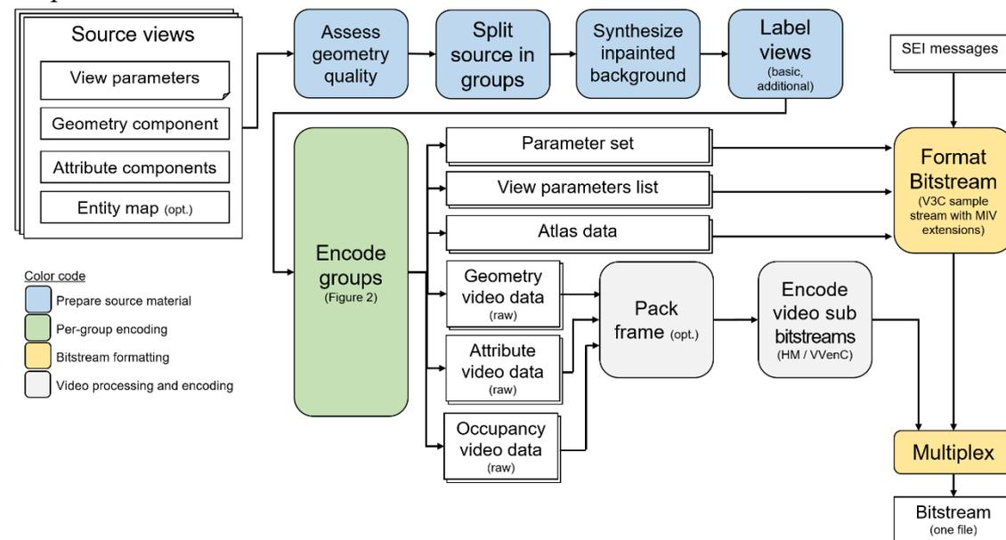
Figure 1: Top-level diagram of the TMIV group-based encoder
