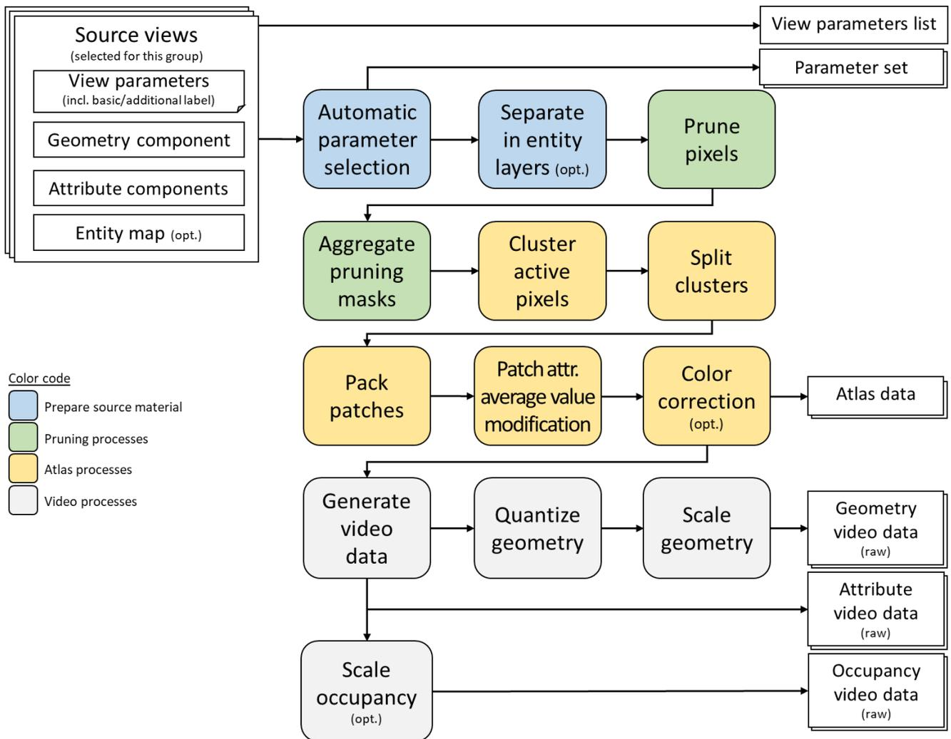
Figure 2: Top-level diagram of the TMIV single-group encoder
