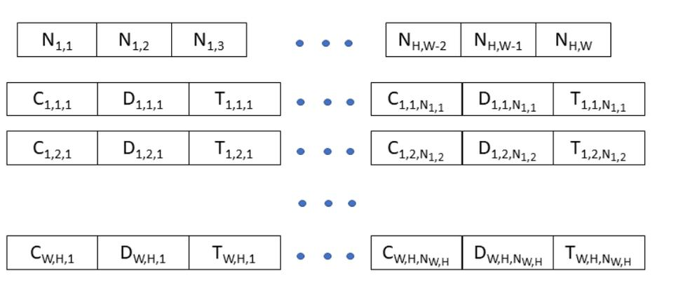
**Figure 32: MPI packed compressed storage (PCS) layout.**
