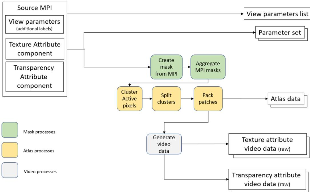
Figure 33: Top-level diagram of the TMIV MPI encoder
