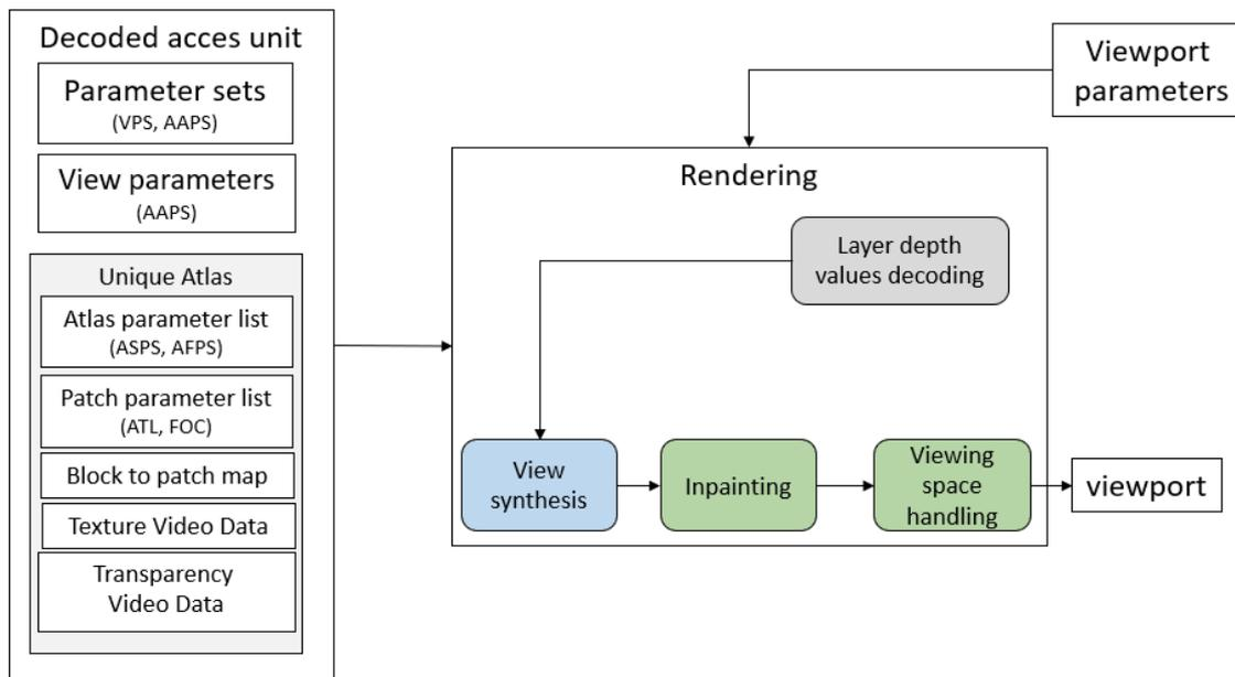
Figure 43: Process flow for TMIV MPI renderer
