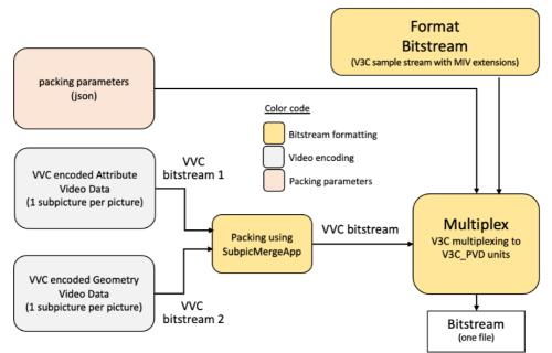
Figure 25: Encoding of texture and geometry components into one packed video sub-bitstream
