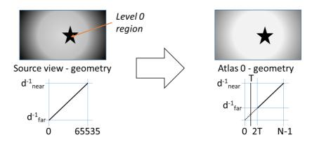
Figure 23: When the source material has invalid geometry values, the geometry coder not only performs u(16) to u(10) or u(9) scaling, but it also sets the geometry threshold to a configurated value (T) and the normalized disparity range is modified such that value 2T corresponds to the far geometry; N = 1024 if the geometry has a good quality (§4.2.5) and 512 otherwise
