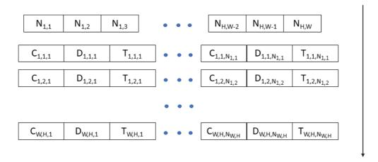
Figure 30: MPI packed compressed storage (PCS) layout.
