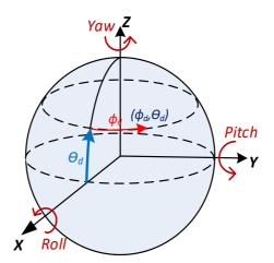
Figure 42: OMAF coordinate system illustrating the directions of positional and rotational units
