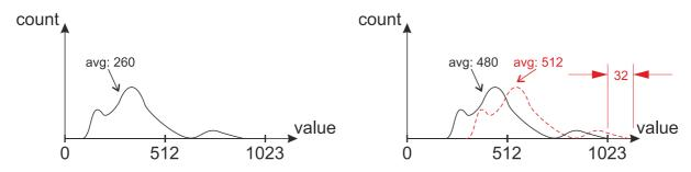
Figure 20: Histogram of an attribute component of a patch: before (left) and after (right) average value modification (overflow avoiding)
