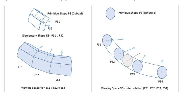
Figure 40: Illustration of VS creation with additive CSG (left) and interpolation (right)
