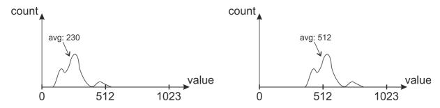
Figure 19: Histogram of an attribute component of a patch: before (left) and after (right) average value modification
