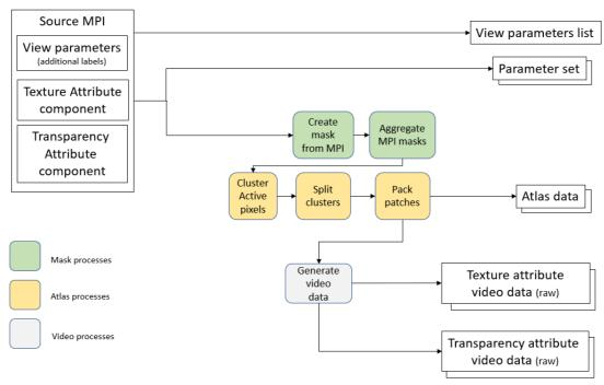
Figure 31: Top-level diagram of the TMIV MPI encoder
