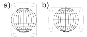
Figure 38: Cylinders used in the projection of a sphere on a flat image in a) equirectangular projection and b) transverse equirectangular projection
