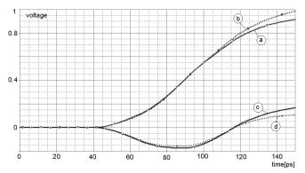
Fig. 5. Ramp response ( $T_r$ =50ps) of the coupled interconnects (Fig.2) a) aggressor line obtained from SPICE b) aggressor line computed from (13), c) victim line computed from SPICE, d) victim line computed from (13)
