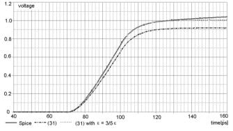
Fig. 4. Ramp response of the single interconnect with parameters taken from [4]. The transmission line model parameters:  $R_t=25\Omega$ ,  $L_t=5nH$ ,  $C_t=1pF$ ,  $C_0=0.1pF$ ,  $R_w=25\Omega$ ,  $T_r=30ps$ .
