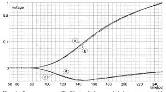
Fig. 6. Ramp response ( $T_r$ =50ps) of the coupled interconnects with parameters taken from [4]. The transmission line model parameters:  $R_t$ =25 $\Omega$ ,  $L_t$ =8nH,  $C_t$ =1pF,  $M_t$ =3,2nH,  $C_m$ =0.1pF,  $C_0$ =1pF,  $R_w$ =25 $\Omega$ . a) aggressor line obtained from SPICE b) aggressor line computed from (13), c) victim line computed from (13)
