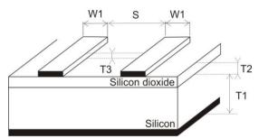
Fig. 2. The symmetrical coupled interconnect structure. Structure dimensions:  $W_1 = 1 \mu m$ ,  $S = 2 \mu m$ ,  $T_1 = 300 \mu m$ ,  $T_2 = 3 \mu m$ ,  $T_3 = 1 \mu m$ , length d=5mm, and the material parameters:  $\epsilon_{Si} = 11.9$ ,  $\epsilon_{Si02} = 4.2$ ,  $\sigma_{Si} = 10000[S/m]$  and  $\sigma_{Cu} = 2.73e + 7[S/m]$ .
