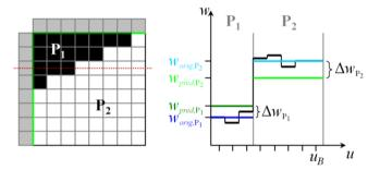
Figure 20: CPVs of block partitions: CPV prediction from adjacent samples of neighbouring blocks (left) and cross section of block (right), showing relation between different CPV types.
