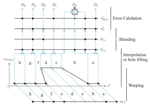
Figure 29: Example for the dependencies between input, intermediate and output signals of the rendering or error calculation step.
