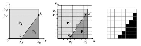
Figure 18: Wedgelet partition of a block: continuous (left) and discrete signal space (middle) with corresponding partition pattern (right).
