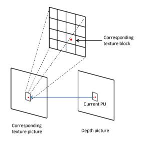
Figure 24: The derivation of corresponding texture block
