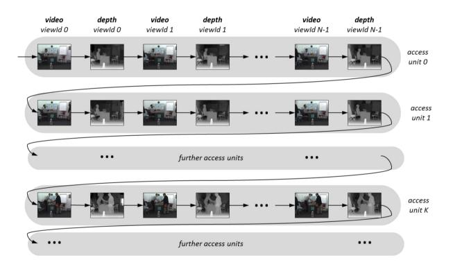
Figure 2: Access unit structure and coding order of view components.
