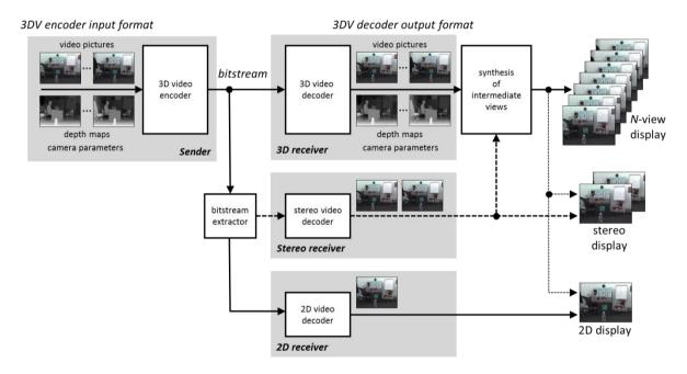
Figure 1: Overview of the system structure and the data format for the transmission of 3D video.
