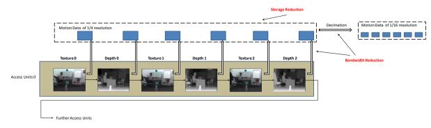
Figure 27: Progressive motion compression for motion data buffer reduction.
