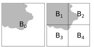
Figure 32: Distortion calculation on different tree depths. Renderable samples (gray shaded) are not taken into account.
