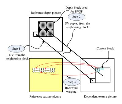
Figure 16: Illustration of the VSP scheme with the neighboring block disparity vector
