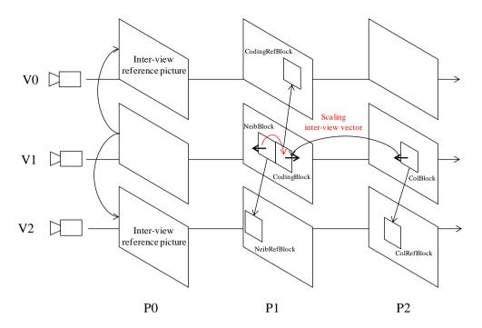
Figure 11: Inter-view motion vector scaling in TMVP
