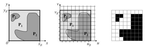
Figure 19: Contour partition of a block: continuous (left) and discrete signal space (middle) with corresponding partition pattern (right).
