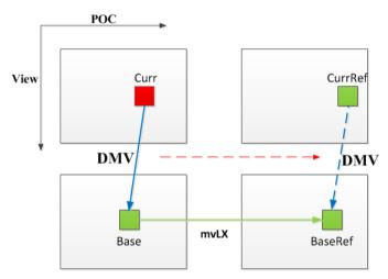
Figure 14. Prediction structure of ARP for inter-view residual.
