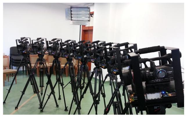
Figure 5. Multi-camera setup used in production of "Poznan Blocks" test sequence.
