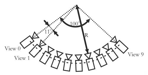
Figure 3. Circular camera setup used in the experiments reported in this documet.
