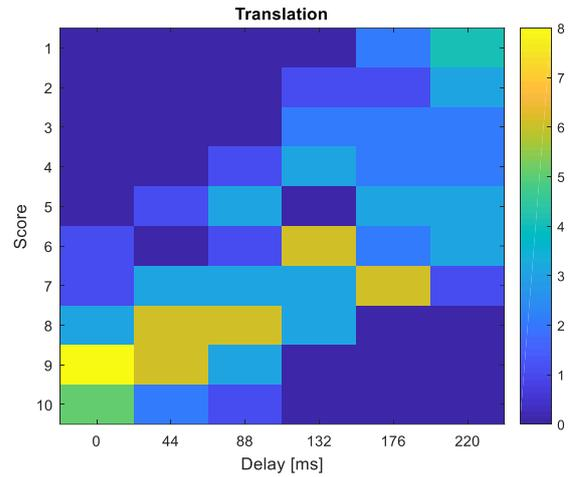
Fig. 8. The histogram of score distribution for different translation delays (ClassroomVideo test sequence).
