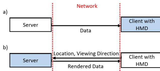
Fig. 1. Basic server and user data exchange models (video processing is performed in blue blocks).
