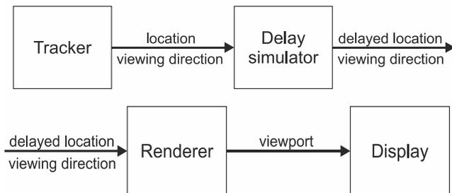
Fig. 5. Data flow in the experiment.
