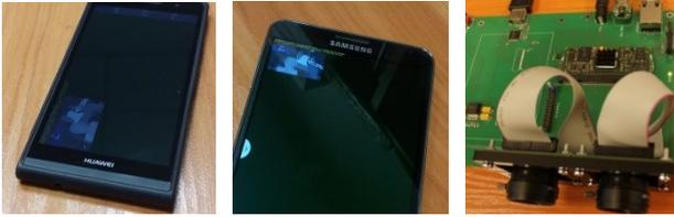
Figure 3. The proposed disparity estimation algorithm implemented on Android mobile devices (Huawei Ascend P6, Samsung Galaxy Note 3) and on the processing board developed by the authors equipped with Xilinx Artix-7 FPGA
