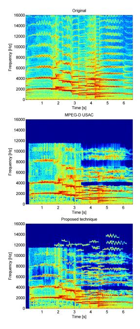
**Fig. 3.** Example spectrograms for signal violin2 and target bit-rate of 16 kb/s, from the top: input signal, full reconstructed signal in the decoder (MPEG-D USAC), full reconstructed signal in the decoder (proposed technique).
