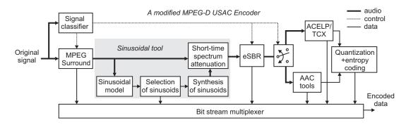
Fig. 1. The modified MPEG-D USAC encoder with additional blocks related to the proposed sinusoidal tool.
