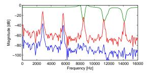
**Fig. 2.** STSA in a single frame:  $X_m(k)$  (red) is attenuated by  $G_m(k)$  (green). The resulting spectrum  $Y_m(k)$  (blue) is shifted by -20 dB for clarity.
