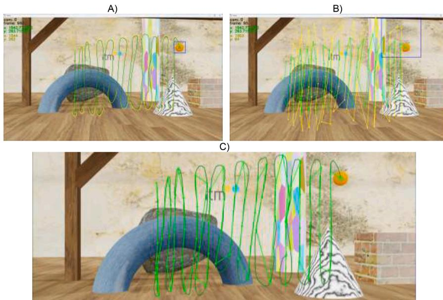
Fig. 3. Tracked marker. Yellow lines: the predicted path of a marker; green lines: the actual path measured by the marker tracker algorithm; blue rectangle: area in which the marker is being searched for; A: analysis of consecutive frames of a calibration sequence, B: analysis of every 10th frame of a calibration sequence, C: comparison of detected marker positions in A (dark green line) and B (light green line) – the curves overlap every 10th frame (light green dots).
