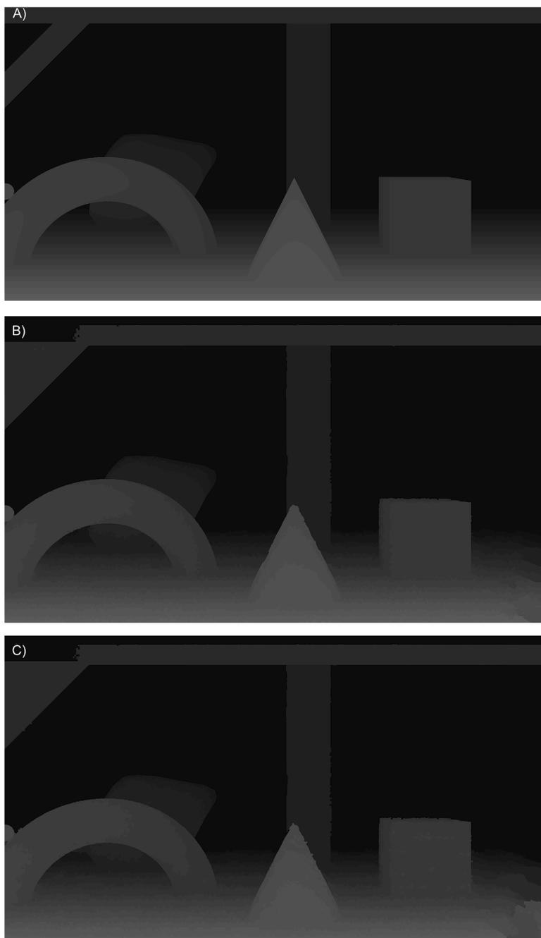
**Fig. 4.** Depth maps for view 6: A) rendered by Blender, B) estimated using exact camera parameters, C) estimated using calibrated camera parameters. The contrast of images was increased to highlight differences. Note that the quality of B is worse than for A because of imperfection of a depth estimation algorithm which cannot perfectly estimate depth for some parts of the scene (especially for areas acquired by a single camera (e.g., left top part of the view)).
