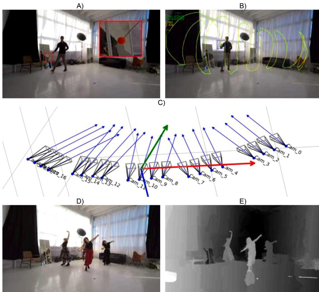
**Fig. 5.** Using ECPC for natural sequence. A: single frame of calibration sequence, B: tracked marker, C: visualization of multicamera system (based on estimated extrinsic parameters), D: single frame of the sequence, E: estimated depth map.
