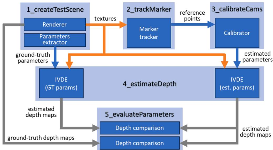
Fig. 1. The general scheme of the ECPC software.
