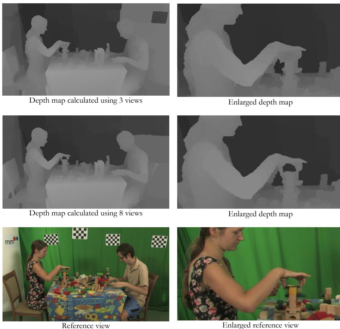
Fig. 6.6. The comparison of depth maps calculated for the different number of input views for the “Poznań Blocks” sequence.
