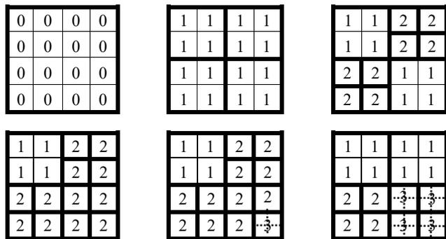
Fig 1. Examples of CTU partitioning schemes based on partitioning depth levels (0..3) in LLCU blocks. Please note that LLCU blocks with level 3 are partitioned even furtherly (deeper – dotted line), than the grid of the LLCUs (solid bold line).
