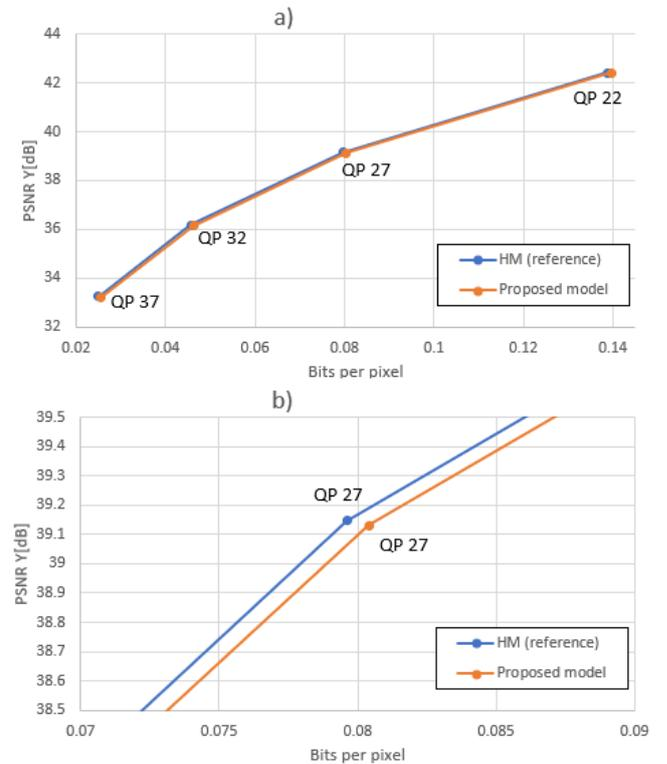
Fig 3. RD-curves for HM (reference) and proposed model. a) RD-curves are almost identical overlaps b) Zoom in on the RD-curves for QP=27 point. A small difference between curves is visible
