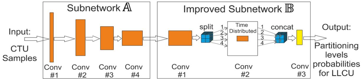
Fig. 2. The proposed architecture of artificial neural network in a straightforward approach, with improved subnetwork  $\mathbb{B}$ , as compared to [1].
