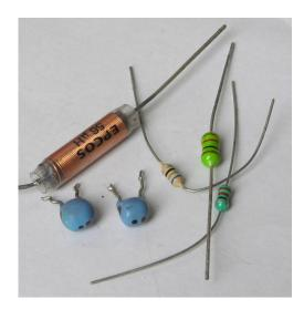
Figure 2.28 Low current inductors. The EPCOS one on the left is for higher current – a few amperes.
