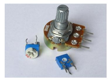
Figure 2.12 Single turn potentiometers
