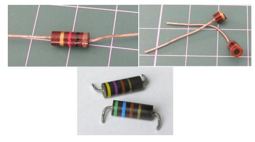
Figure 2.4 Carbon volume resistors
