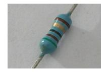
Figure 2.8 An example of a resistor with 5 stripes
