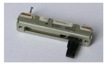
Figure 2.14 Slide potentiometer
