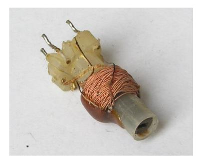
Figure 2.32 Variable inductor with screwed-in core
