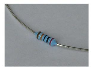
Figure 2.6 Metal film resistor
