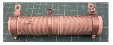
Figure 2.7 Wire wound resistor
