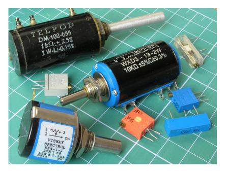
Figure 2.13 Multi-turn potentiometers
