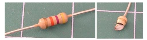
Figure 2.5 Carbon film resistor
